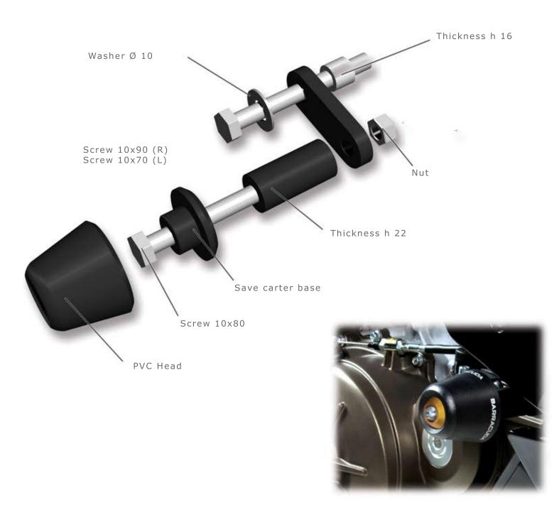
SEARCH AND FIND THE FIXING POINT ON THE MOTORBIKE, USE THE SPECIFIC THICKNESS AND BOLTS LIKE DESCRIBED IN THE PICTURE (SO YOU CAN GET THE RIGHT PROMINENCE FROM THE MOTORBIKE). FIX THE PVC HEAD AFTER FIXED AND TIGHTEN ALL THE KIT ONLY.
