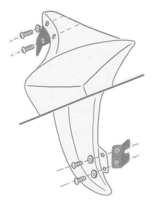
MOUNT THE BRACKETS ON THE BARRACUDA AIR CONTROL LIKE IN THE PICTURE. FIX THE BARRACUDA AIR CONTROL ON THE MOTORBIKE USING THE ORIGINAL SCREW IN THE UPPER PART OF RADIATOR AND THE 8X16 SCREW IN THE DOWN PART THE RESPECTIVE NUT.
