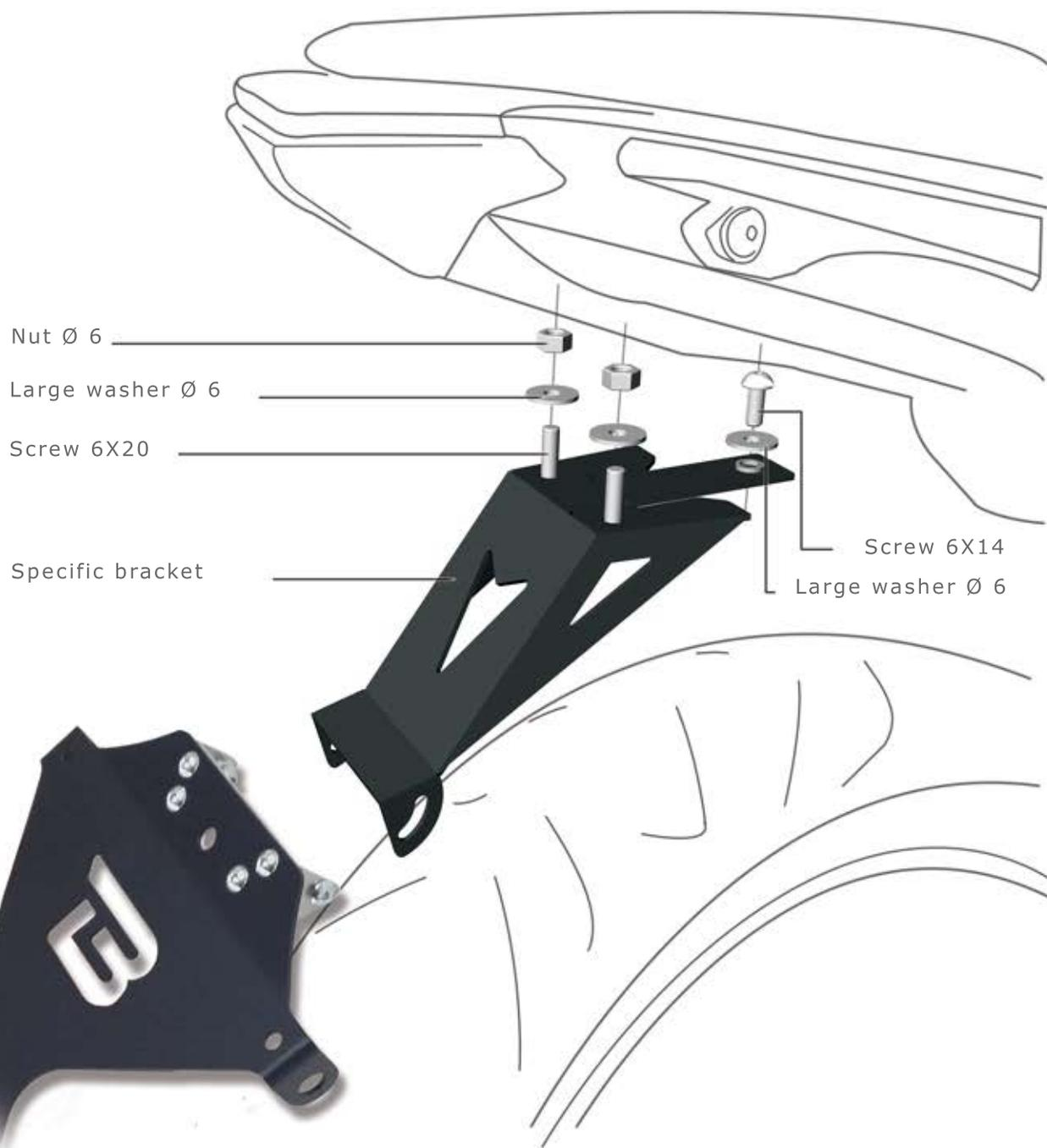
REMOVE THE ORIGINAL LICENCE PLATE. FIX THE BARRACUDA SPECIFIC BRACKET USING THE SCREWS INCLUDED LIKE SHOWN IN THE PICTURE. APPROACH AND FIX THE "X" LICENCE PLATE TO THE INSTALLED BRACKET.
