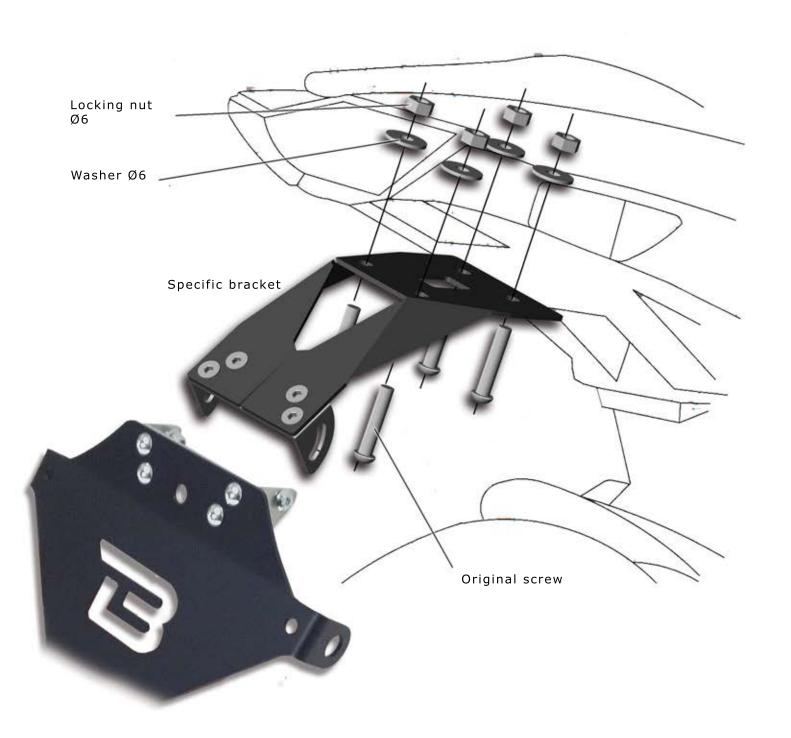
REMOVE THE ORIGINAL LICENCE PLATE. APPLY THE BARRACUDA SPECIFIC BRACKET WITH THE SCREWS LIKE SHOWN IN THE PICTURE. USE THE WASHERS WITH THE LOCKING DIAMETER 6 NUTS INSIDE.
