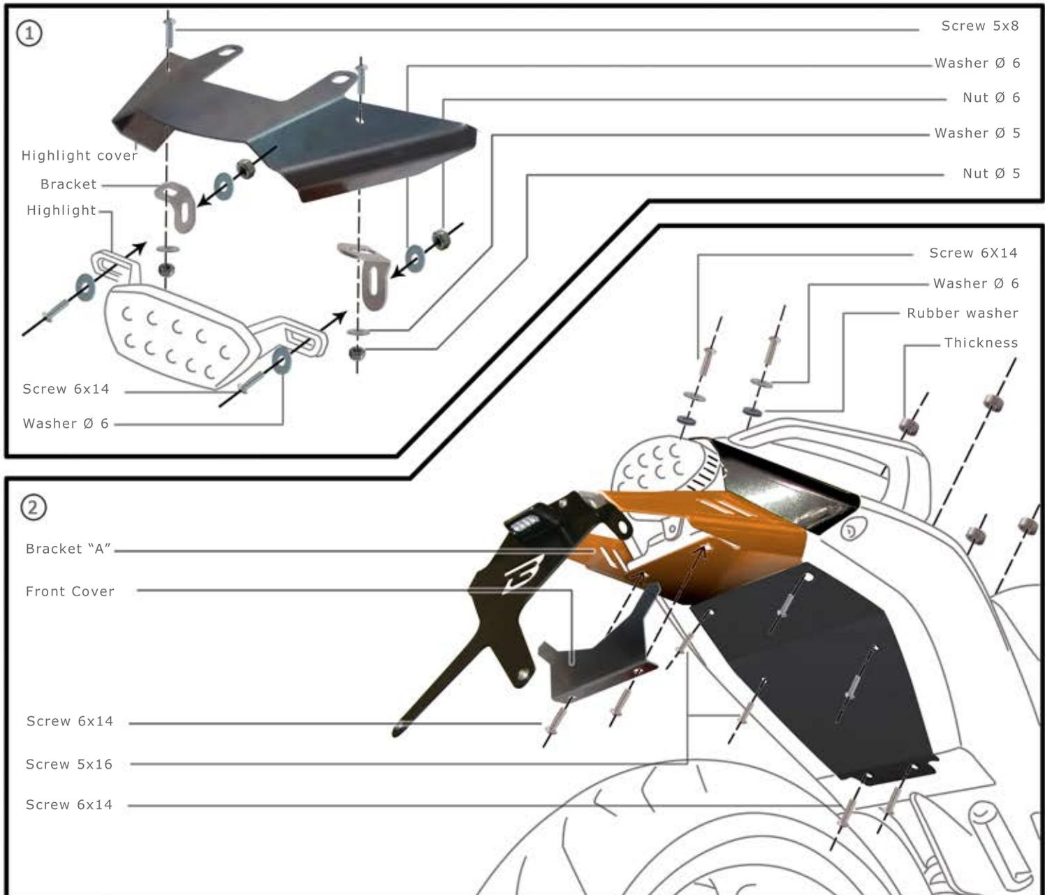
NOTE: WE ADVICE TO TAKE AN INCLINATION NOT EXCEEDING 30° TO AVOID STRUCTURAL POSSIBLE BROKEN
