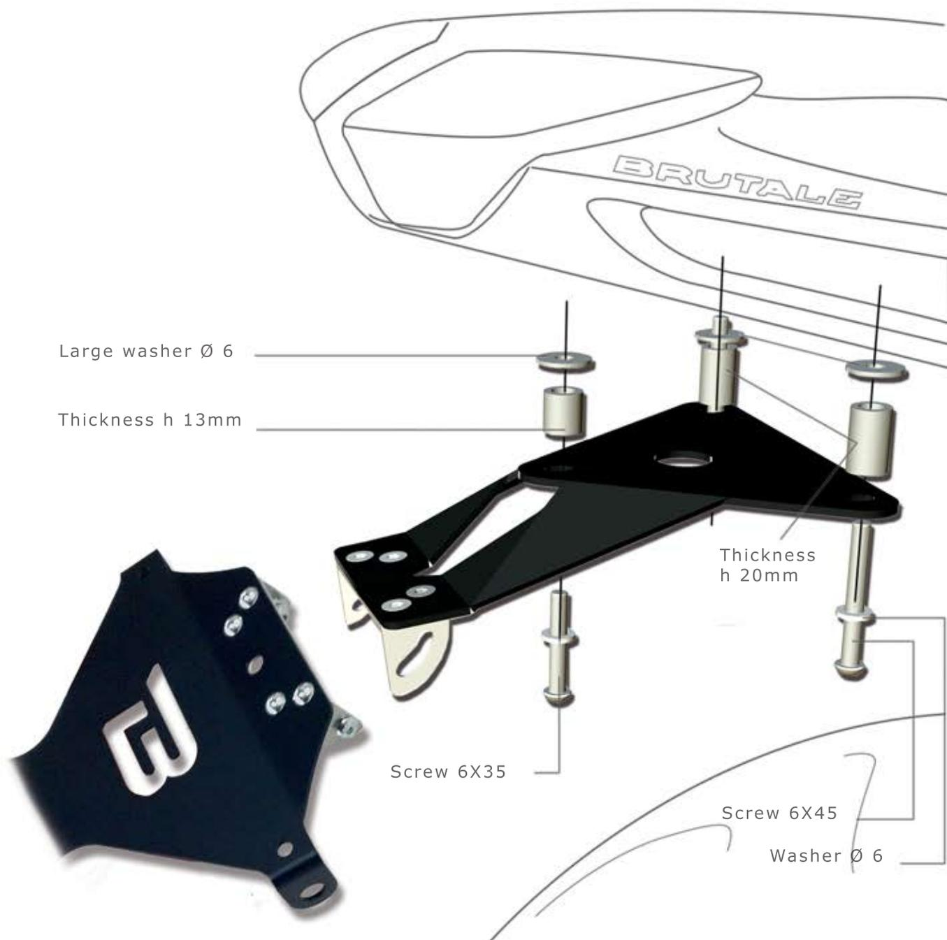
REMOVE THE ORIGINAL LICENCE PLATE FROM MOTORBIKE. APPLY THE BARRACUDA SPECIFIC BRACKET AND FIX IT USING SCREWS AND THICKNESS INCLUDED LIKE SHOWN IN THE PICTURE. APPROACH AND LOCK THE "X" LICENCE PLATE TO THE BRACKET INSTALLED.
