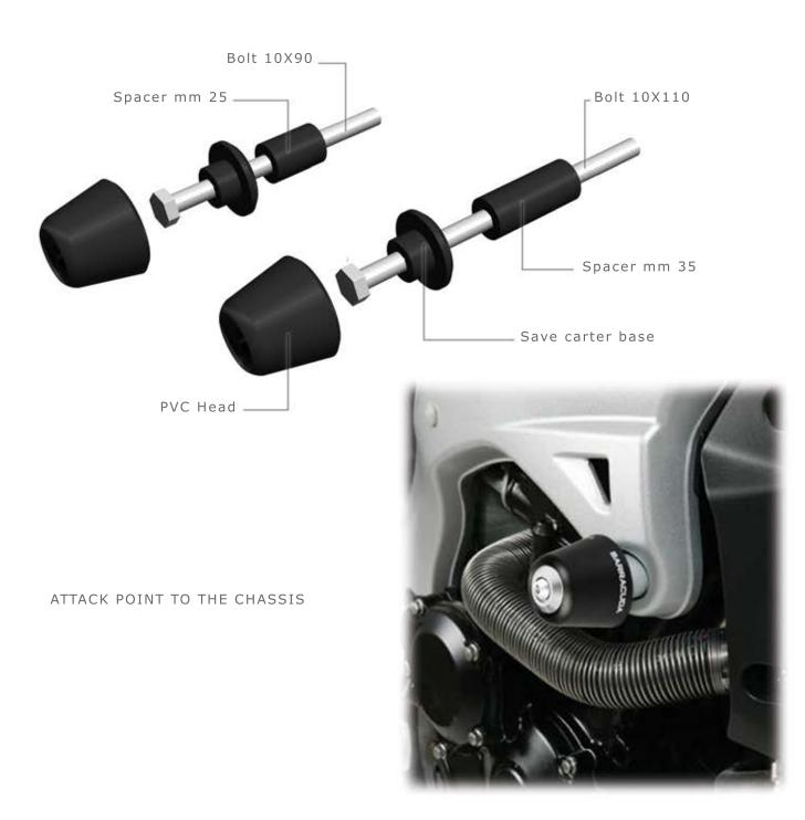
VERIFY THE TWO DIFFERENTS LENGHTS OF THE TWO POINT OF FIXING BEFORE THE MOUNTING PRO-CESS.
