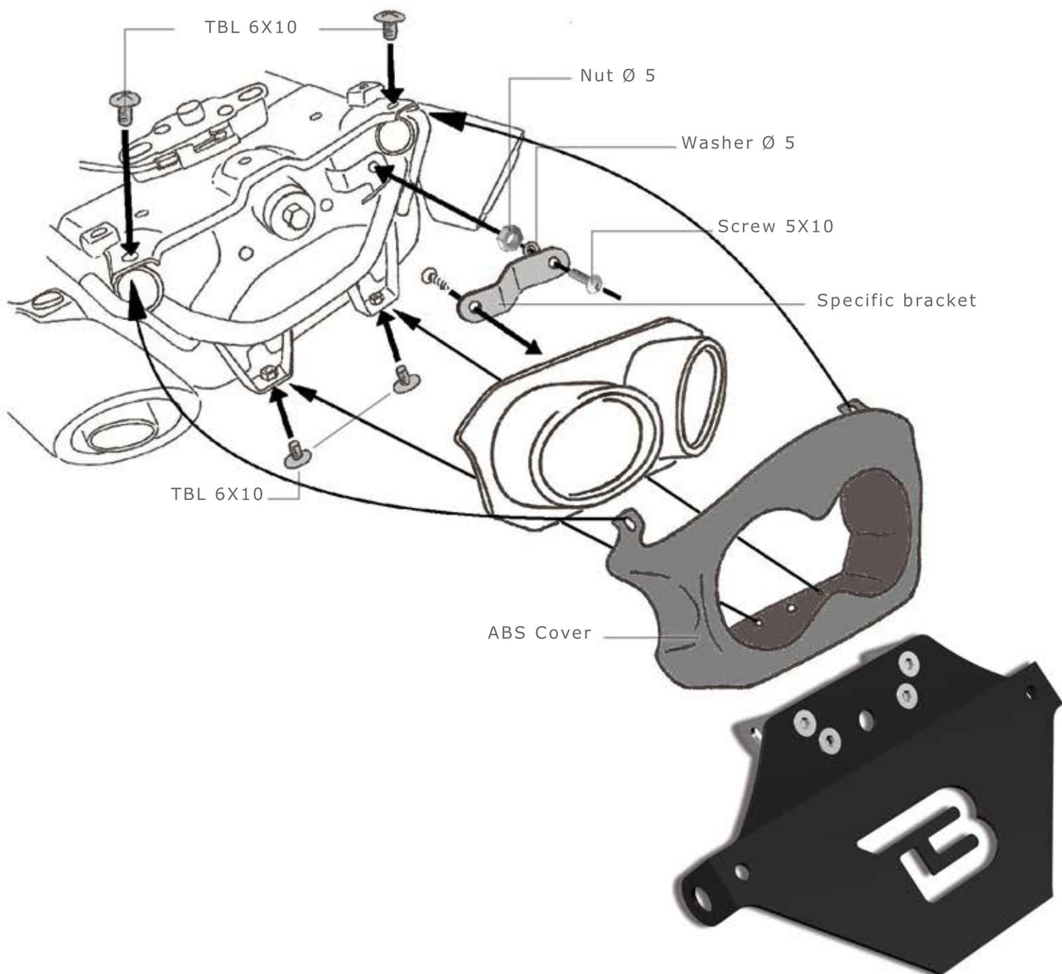
REMOVE THE ORIGINAL LICENCE PLATE FROM THE MOTORBIKE. APPLY THE ABS COVER LIKE DESCRIBED IN THE PICTURE AND THAN APPROACH THE "X" LICENCE PLATE BARRACUDA
