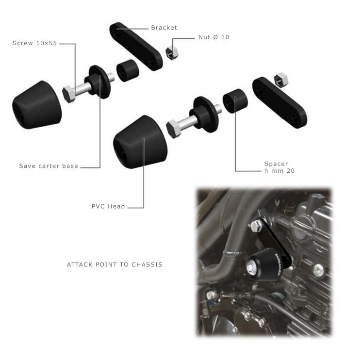
SEARCH AND FIND THE FIXING POINT ON THE MOTORBIKE BEFORE START TO MOUNTAIN, USE THE SPE-CIFIC THICKNESS AND BOLTS LIKE DESCRIBED IN THE PICTURE (SO YOU CAN GET THE RIGHT PROMI-NENCE FROM THE MOTORBIKE).
