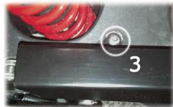
REMOVE THE REAR FENDER AND UNSCREW THE FIXING
