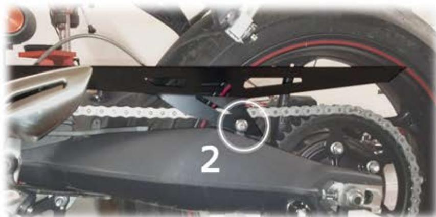
UNINSTALL THE ORIGINAL CHAIN COVER AND REAR FENDER REMOVING THE FIXING SCREWS ON THE
