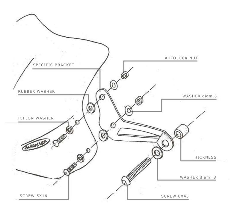
INSTALL THE WINDSHIELD/SCREEN LIKE DESCRIBED IN THE PICTURE. PUT THE TEFLON WASHERS BETWEEN THE HEAD OF SCREW AND THE WINDHSIELD. DON'T LOCK TOO MUCH THE AUTOLOCK NUTS DIAMETER 5 TO AVOID DAMAGES
