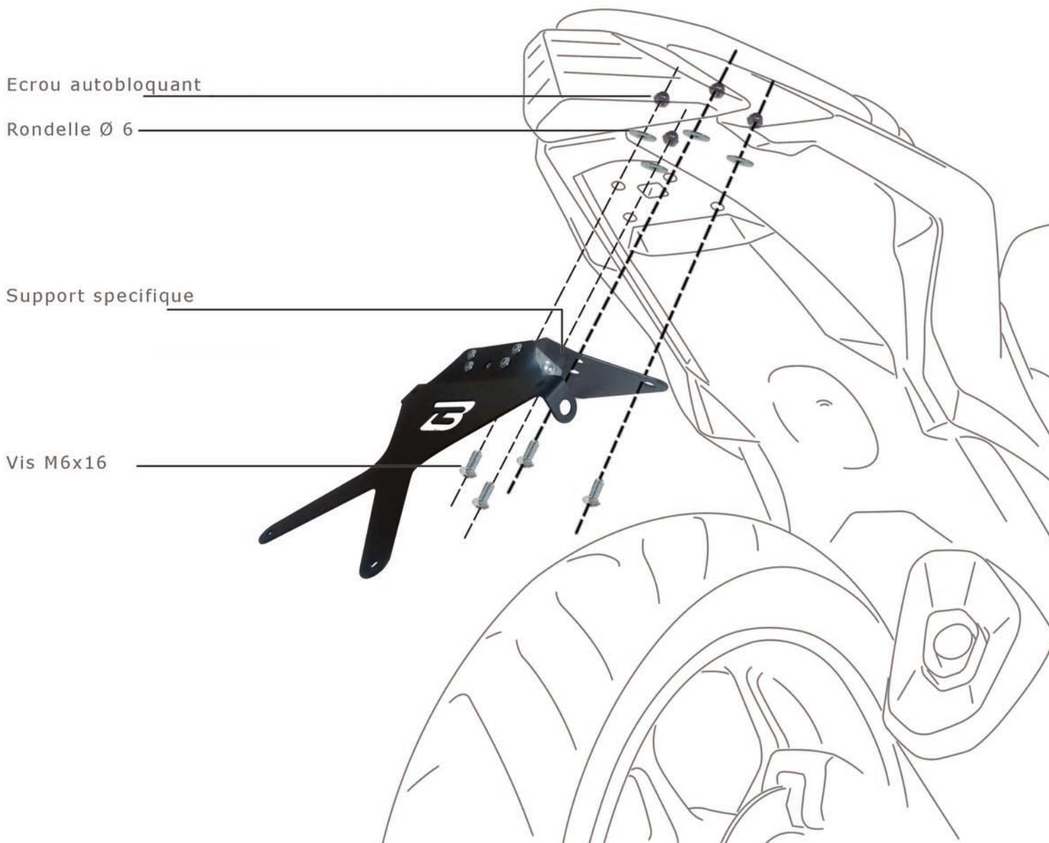
NOTE: LA PLAQUE DOIT ETRE ORIENTÉE A 30° PAR RAPPORT À UNE PERPENDICULAIRE AU SOL.
