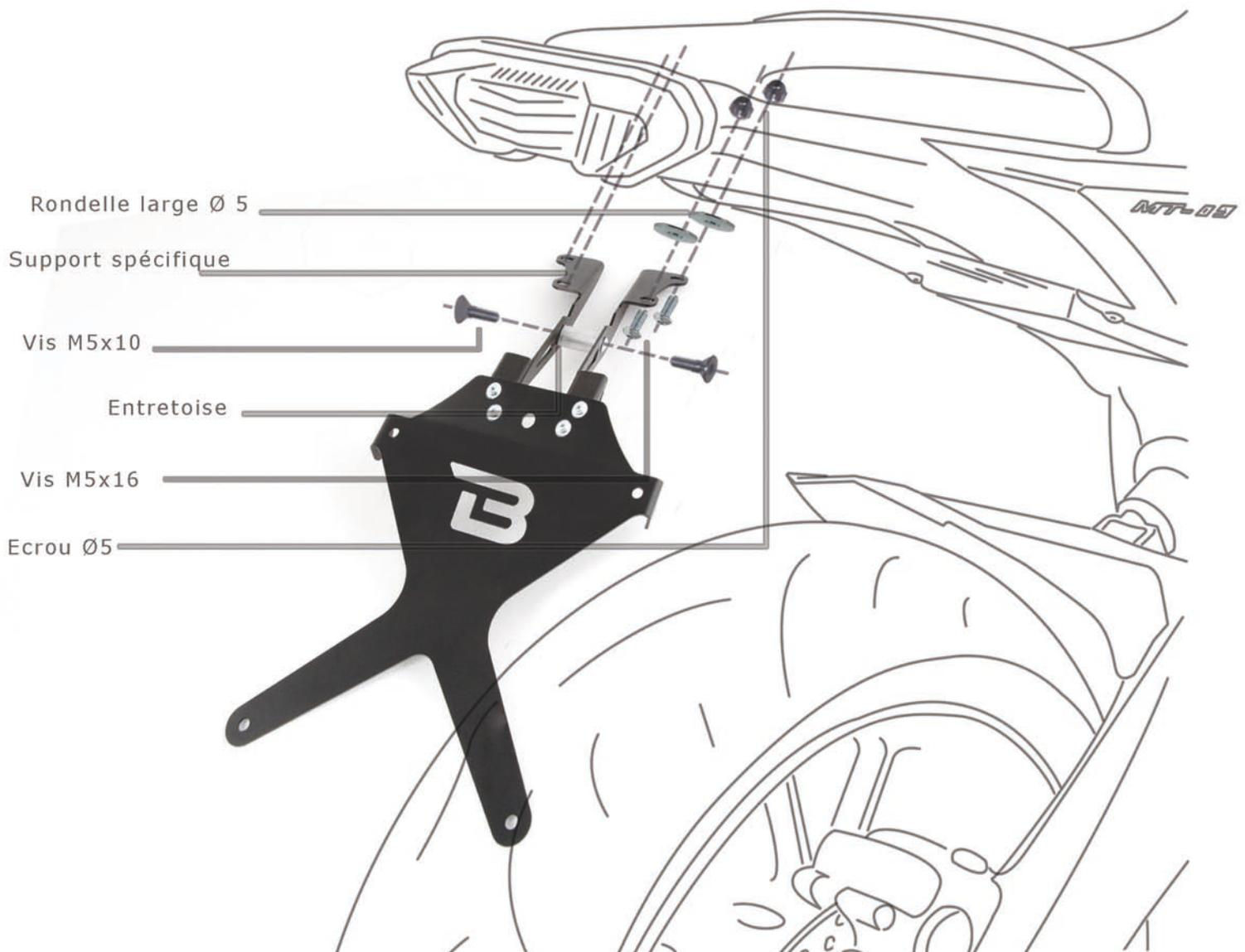
L'INCLINAISON DE LA PLAQUE DOIT ETRE DE 30° PAR RAPPORT A UNE PERPENDICULAIRE AU SOL.
